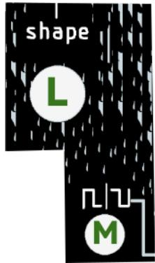
Shaper is essentially a CV controlled crossfader which can smoothly fade between two signals, allowing for a wide combination of waveshapes. The balance between the two signals can be adjusted with Shape knob (L) or with modulation applied to the Shape CV input (8).
