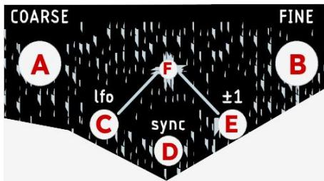
LFO switch (C) determines if Occult will operate as VCO (audio rate) or LFO. In LFO mode (up position) Occult allows for slow cycles which make it a great complex modulation source. In VCO mode it can reach from 20hz to above 20khz.
