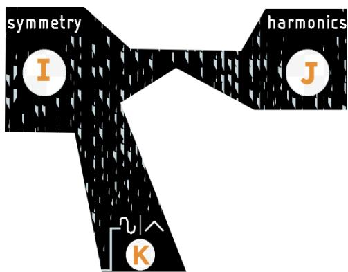
Symmetry knob (I) controls the pulse widths of the produced pulses, essentially increasing or decreasing the thresholds of the comparators. Symmetry can be modulated through Symm CV input (7).
