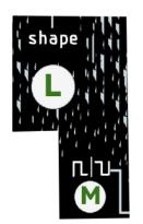
Shaper is essentially a CV controlled crossfader which can smoothly fade between two signals, allowing for a wide combination of waveshapes. The balance between the two signals can be adjusted with Shape knob (L) or with modulation applied to the Shape CV input (8).
